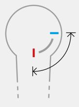
The optimal lever position for energy-efficient warm water is in the middle and allows an intuitive correct operation (ideal using temperatures  $35 \,^{\circ}$ C,  $38 \,^{\circ}$ C or maximum  $45 \,^{\circ}$ C).
